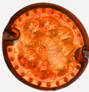
Front Combination Lamp Assembly consisting of Front Position Lamp & Direction Indicator Lamp 9 LED
