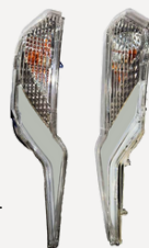
Front Combination Lamp Assembly Consisting of Front Position and Direction Indication Lamp
