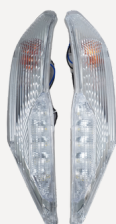
Front Combination Lamp Assembly consisting of Front Position Lamp & Direction Indicator Lamp
